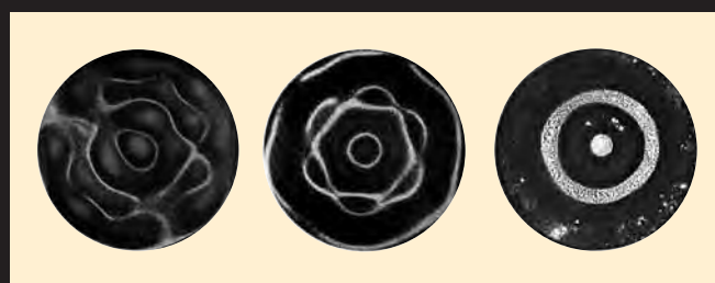
Top: Fig. 2 Ernst F.F. Chladni demonstrates 'nodal patterns' by bowing a small steel plate covered with sand. Bottom: Fig. 3 Sound figures formed on a rubber membrane. Left to right: 'oh', 'ah', and 'oo'. 5 ©2001 MACROmedia Publishing.
